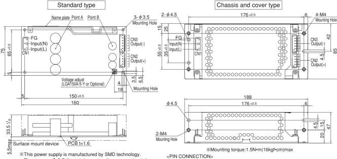
$\ensuremath{\mathrm{\%This}}$  power supply is manufactured by SMD technology. The stress to P.C.B like twisting or bending causes the defect of the unit, so handle the unit with care.
